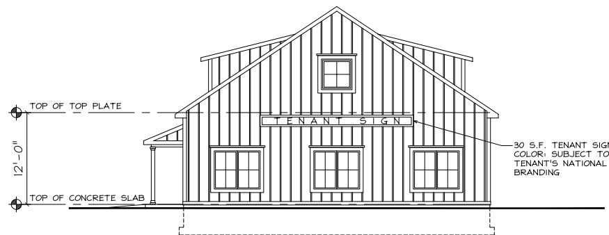
6 EAST BUILDING ELEVATION
