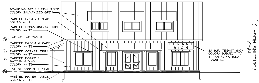
3 SOUTH BUILDING ELEVATION (FACADE)
